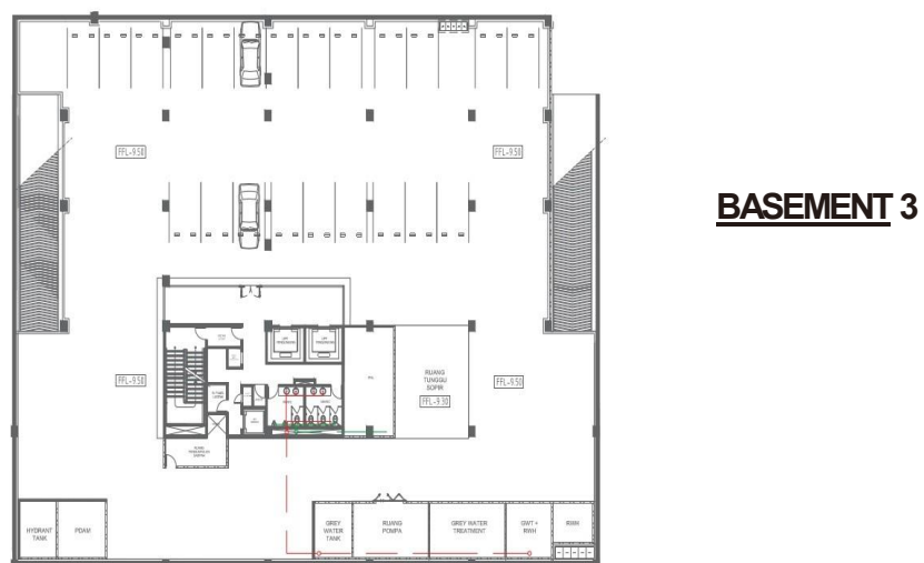
Gambar 4.12 Denah Perletakan Grey water tank dan rain water harvesting
