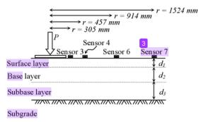
Figure 1. Typical pavement layers and sensor arrangement on the surface of road pavement.
