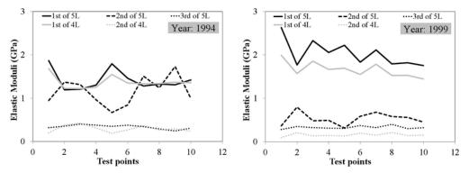
**Figure 4.** Comparion of moduli of a 6-layer road segment A that was simulated as a four-layer (4L) and five-layer (5L) pavement structure.
