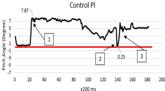
Fig. 8. Pitch angle response of the prototype moving above the water due to disturbance
