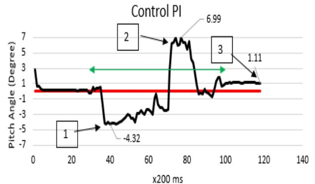
Fig. 6. Pitch angle response of the prototype moving above the ground due to disturbance
