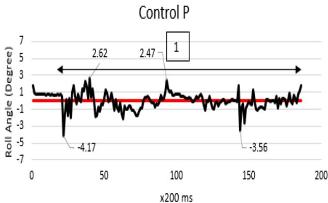
Fig. 7. Roll angle response of the prototype moving above the water due to disturbance
