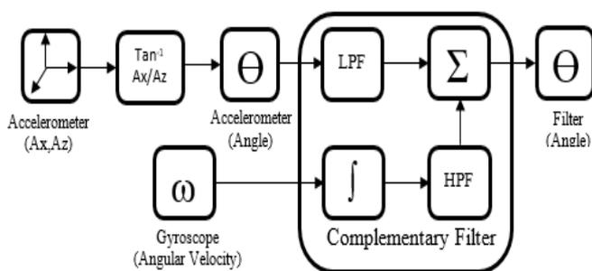
Fig. 4. Complementary filter diagram of rotation angle.
