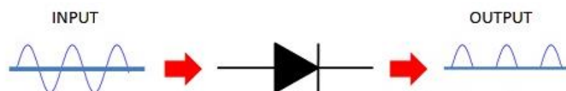
Gambar 2. 22 Prinsip Kerja Dioda [13]
