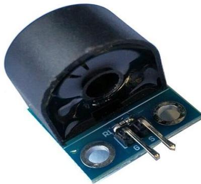
**Gambar 2.20** Sensor ZMCT103C<sup>[5]</sup>
