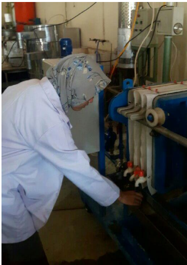
Gambar 9. Pengoprasian alat filter press
