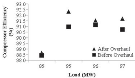
Fig. 1. Compressor efficiency versus load.
