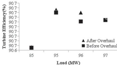
Fig. 2. Turbine efficiency versus load.
