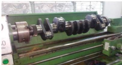
(a). Crankshaft on the lathe machine
