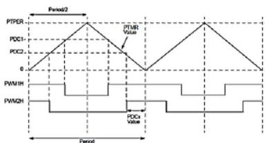
Gambar 7. Diagram PWM center-aligned mode
