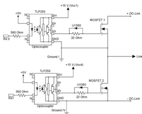
Gambar 2. Rangkaian MOSFET Driver TLP250
