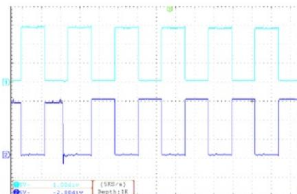
Gambar 15. Output *optocoupler* TLP250 PWM1L & PWM1H
