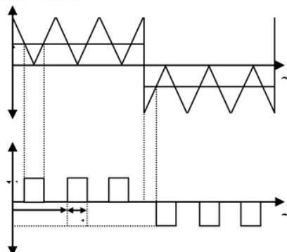
Gambar 4. Uniform Pulse-Width Modulation (UPWM)
