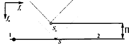
Fig. 1 Contact element in Lagrangian method
