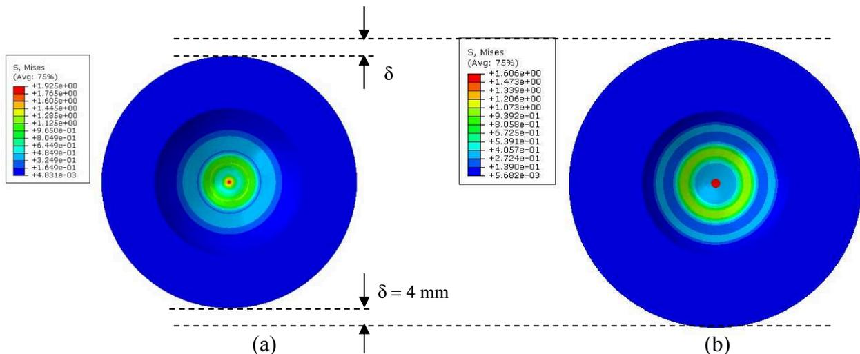
Fig. 4. The von Mises stress distribution of the UHMWPE acetabular liner (top view) for the thickness of: (a) 10 mm and (b) 14 mm.
