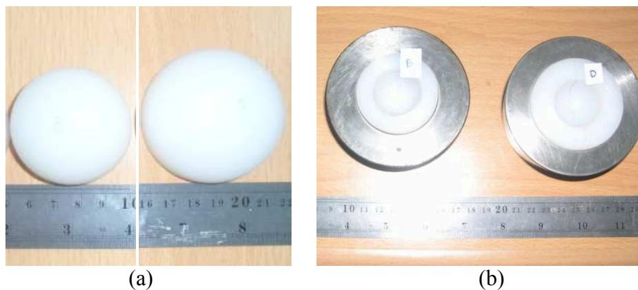
Fig. 1. (a) The two thickness variation of the UHMWPE acetabular liner specimens and (b) the specimens of (a) when it is installed in the holder.
