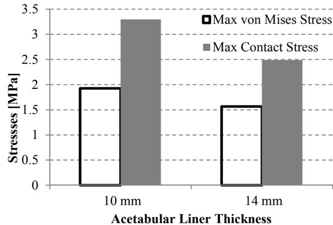
Fig. 5. The maximum of von Mises and contact stresses distribution of the acetabular liner.
