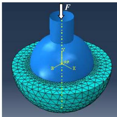
Fig. 2. The finite element contact model between the femoral head and the acetabular liner.
