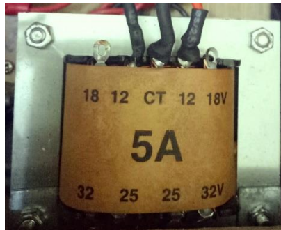
Gambar 2- 34 Transformator Step Down 5A
