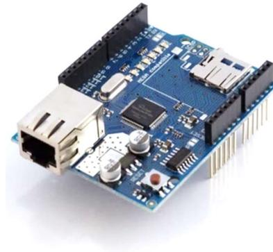
**Gambar 2.32** *Ethernet shield* <sup>[7]</sup>
