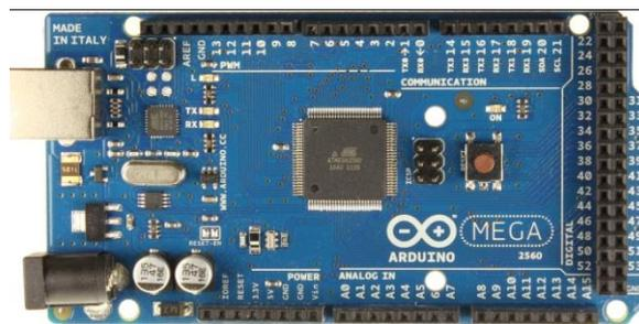
**Gambar 2.5** Arduino Mega 2560 <sup>[9]</sup>
