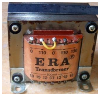
Gambar 2.9 Transformator Step Down 5A
