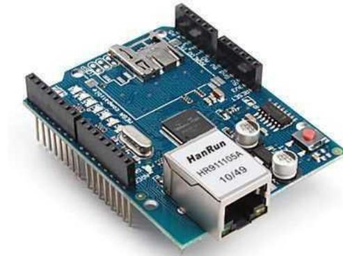
**Gambar 2.44** Ethernet Shield.<sup>[39]</sup>
