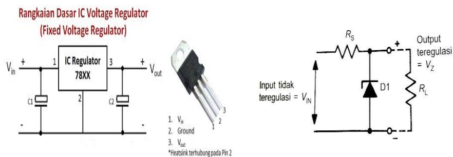
Gambar 2.4 Rangkaian IC Voltage Regulator [1]
