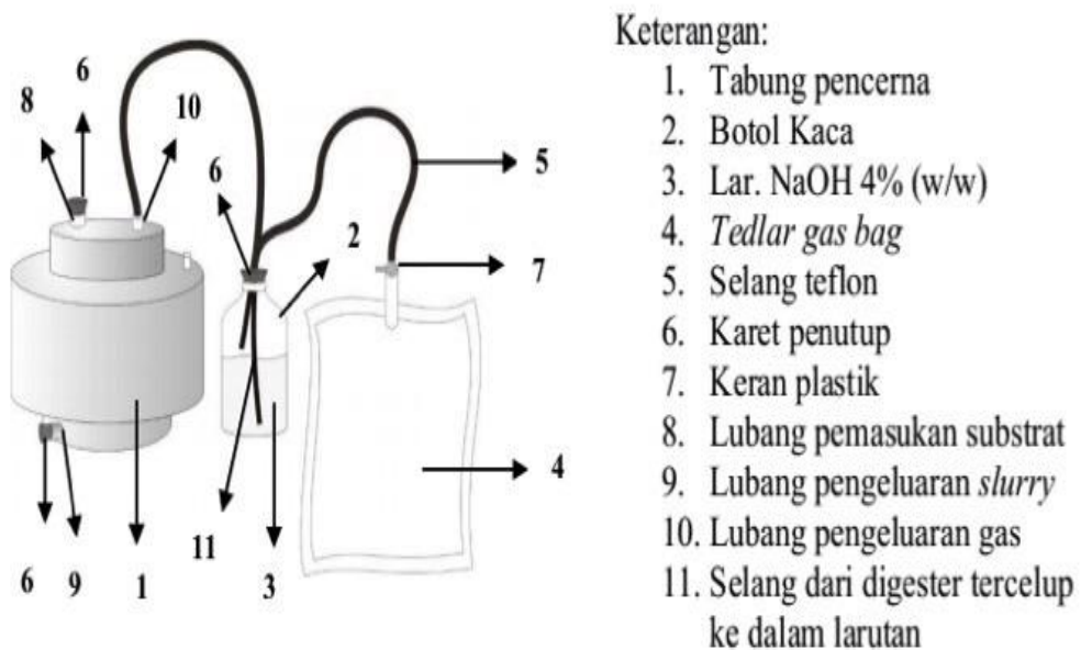
Ilustrasi 1. Digester Tipe Continuous Feeding
