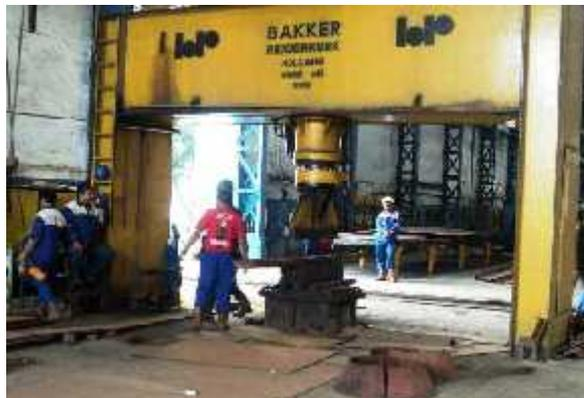
Gambar 2.13 Mesin Bending 3000 kN
