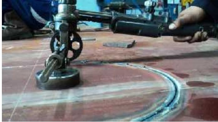
Gambar 2.14 Alat Cutting manual
