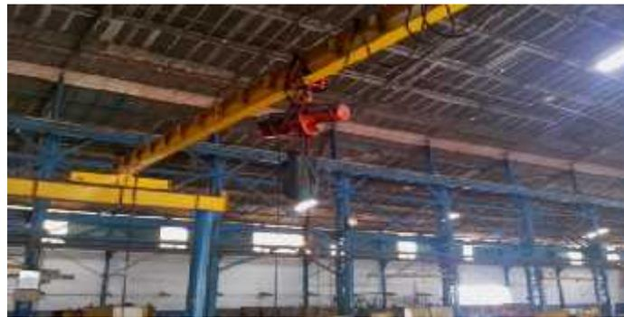
Gambar 2.15 Over Head Traveling Crane 6 ton, 10 ton, dan 16 ton
