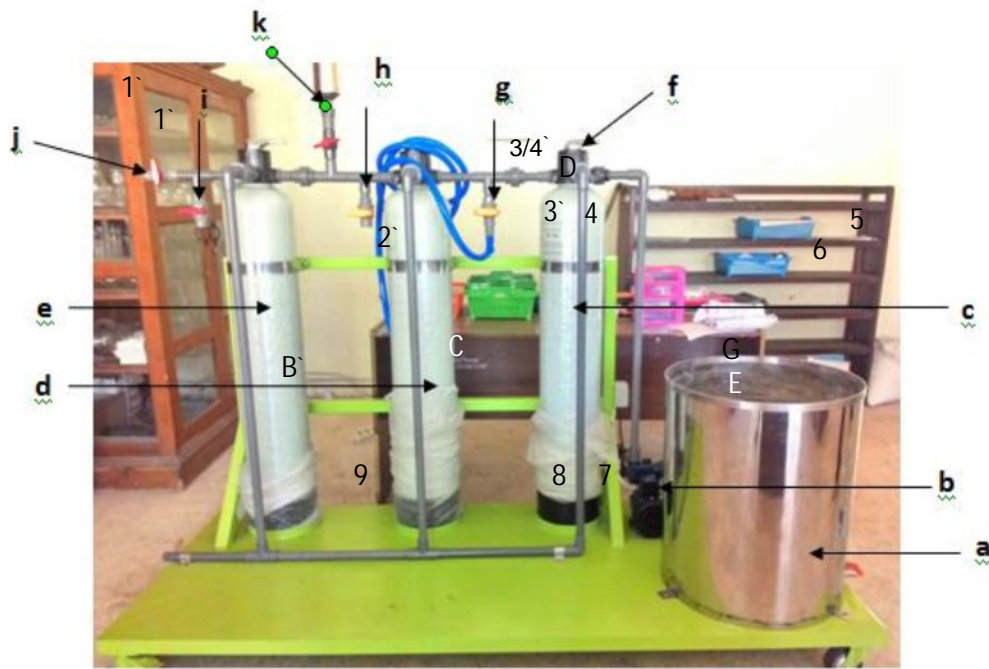
Gambar 2. Skema alat Ion Exchanger
