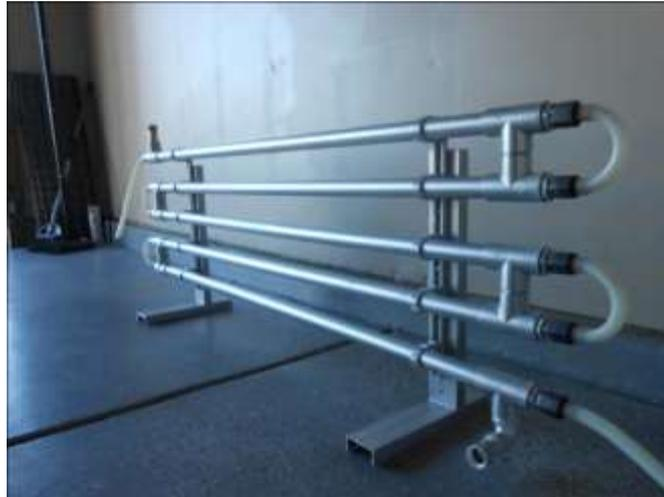
**Gambar 13.** *Double-Pipe Heat Exchangers in Series–Parallel*
