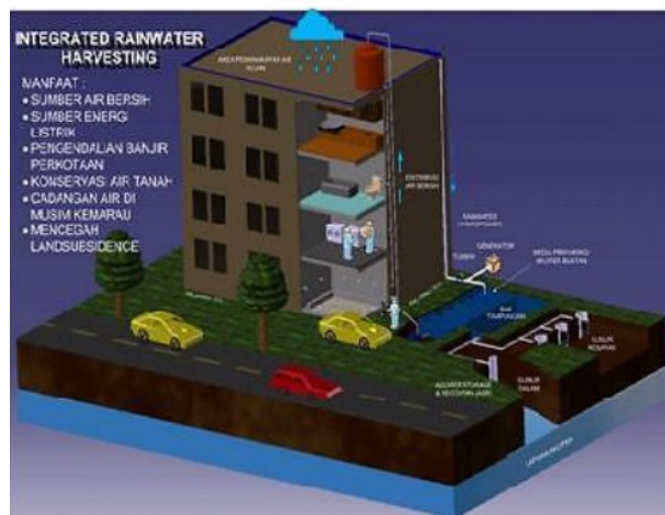
Gambar 5. 11 : Rainwater Harvesting System
