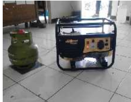
Gambar 3.2 Genset bahan bakar gas
