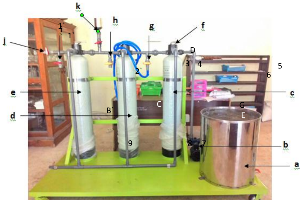
Gambar 2. Skema alat Ion Exchanger
