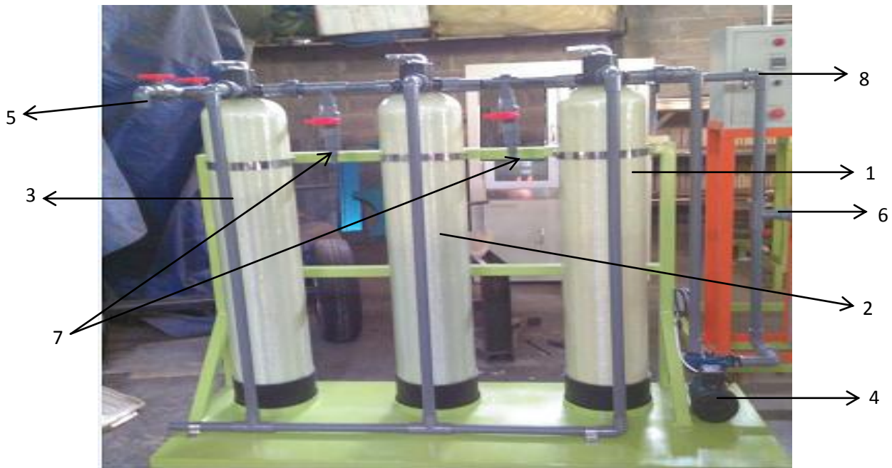
Gambar 4. Skema alat demineralizer
