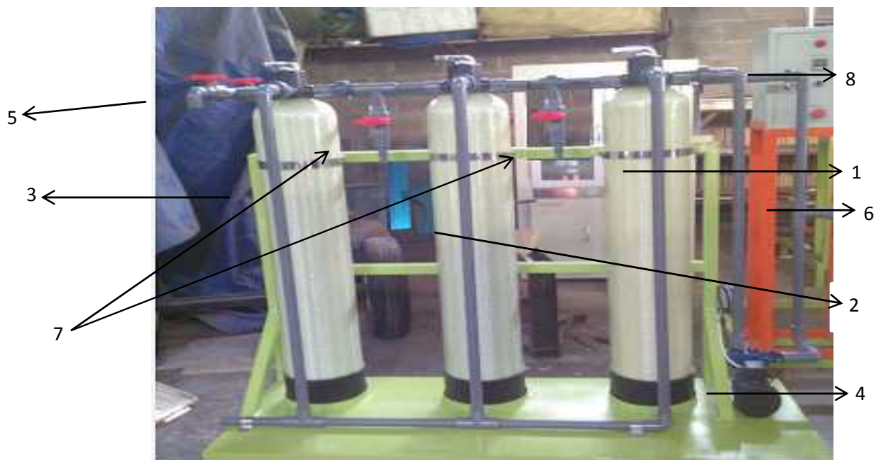
Gambar 1. Skema alat demineralizer
