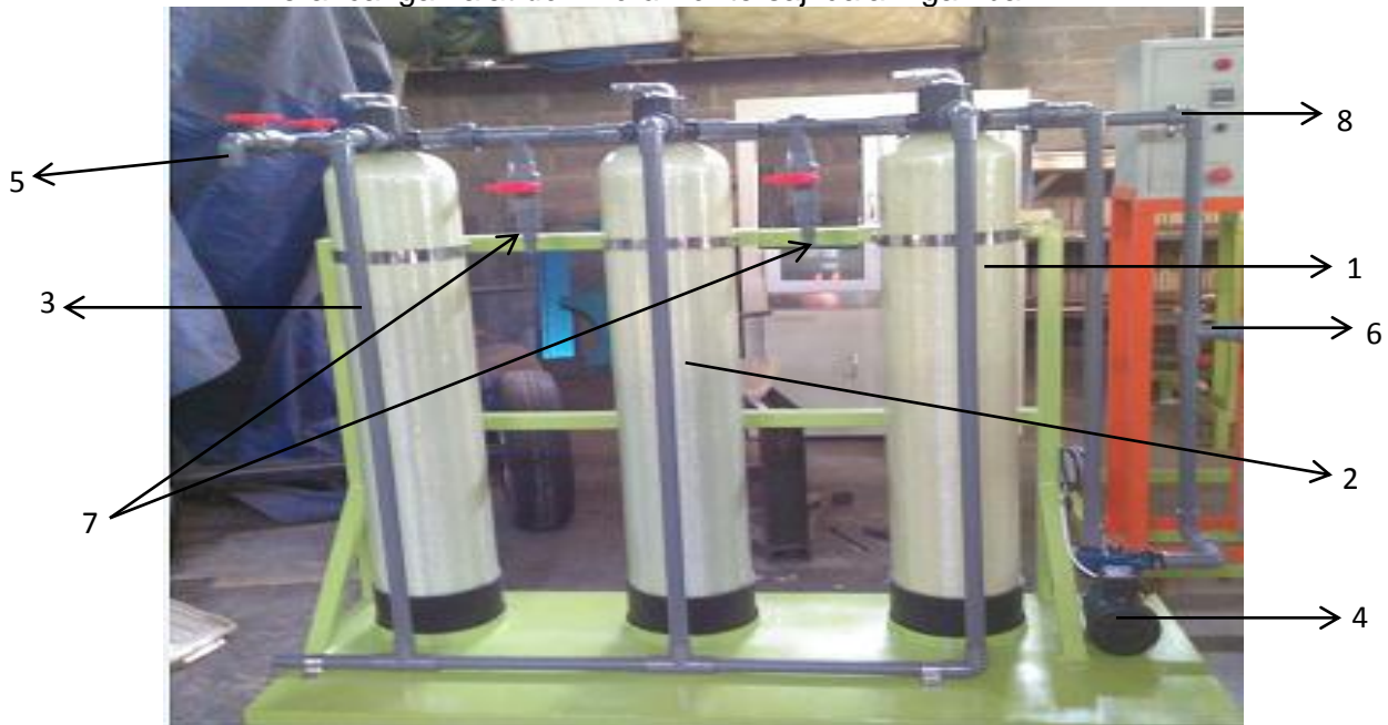
Gambar 1. Skema alat demineralizer
