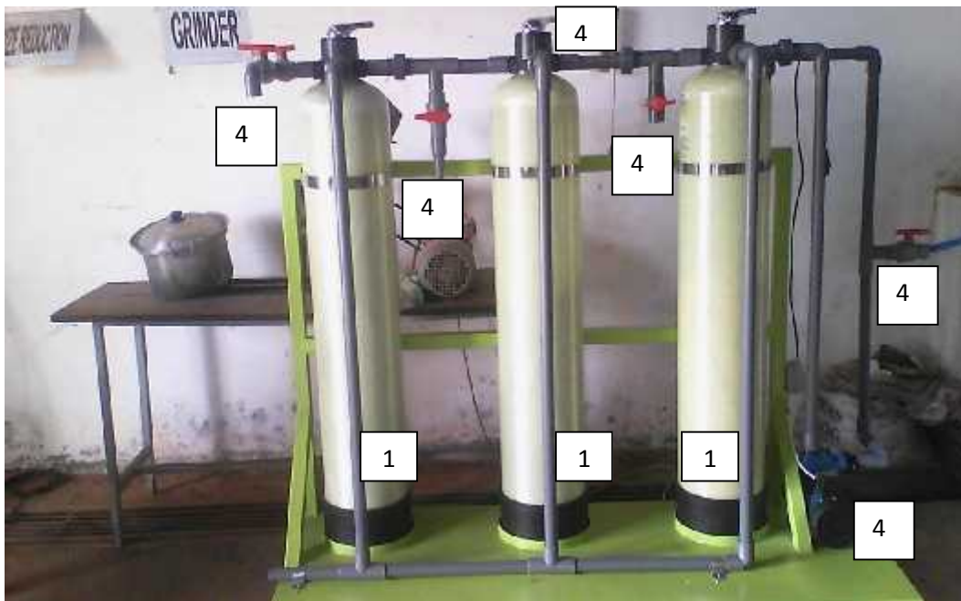
Gambar 1. Skema alat demineralizer
