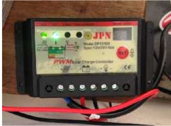
Gambar 2.3. Battery charger controller unit
