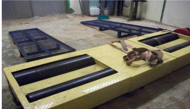
**Gambar 3.6** Chassis Dynamometer
