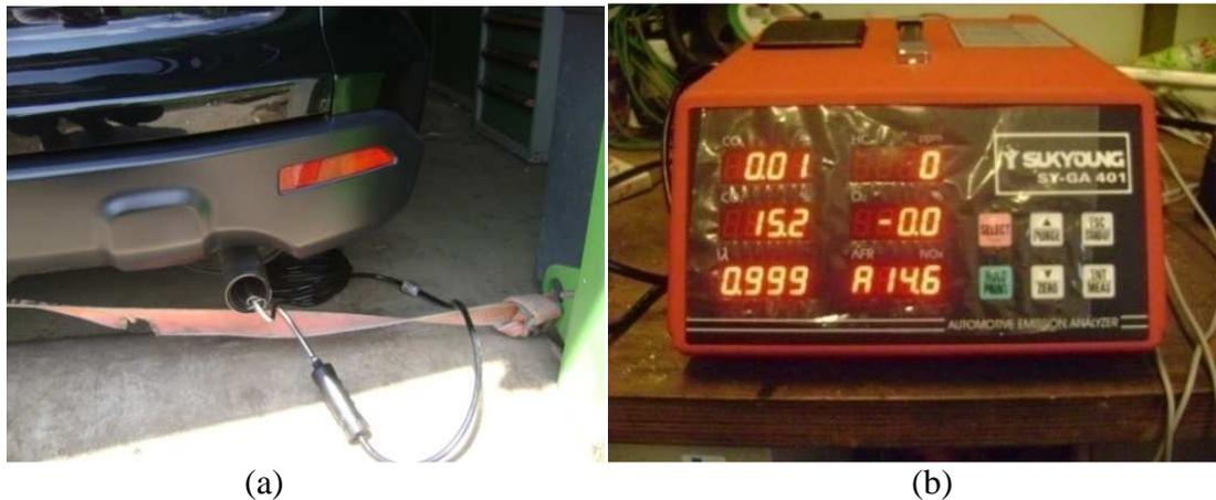
**Gambar 3.11** (a) Memasang probe gas analyzer ke knalpot (b) Gas analyzer
