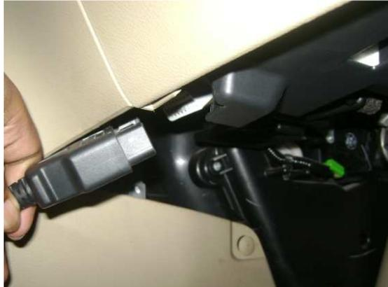
**Gambar 3.10** Pemasangan kabel engine scanner ke soket OBD II
