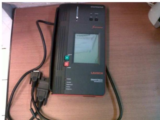
**Gambar 3.4** Engine Scanner Launch
