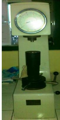
Gambar 3.13. *Rockwell Hardness Tester*.
