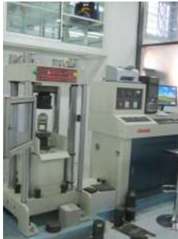
Gambar 3.5 HT-8391PC Computer-Control Servo Hydraulic Concrete Compression Testing Machine
