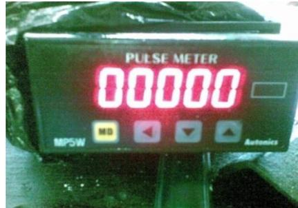
Gambar 3.11 *Display Pulse Meter*
