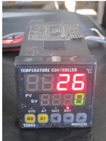
Gambar 3.13 *Display temperature controller*
