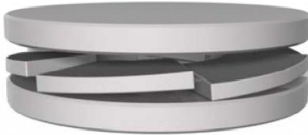
Gambar 2.4. Skema *axial thrust pad bearing* [16]
