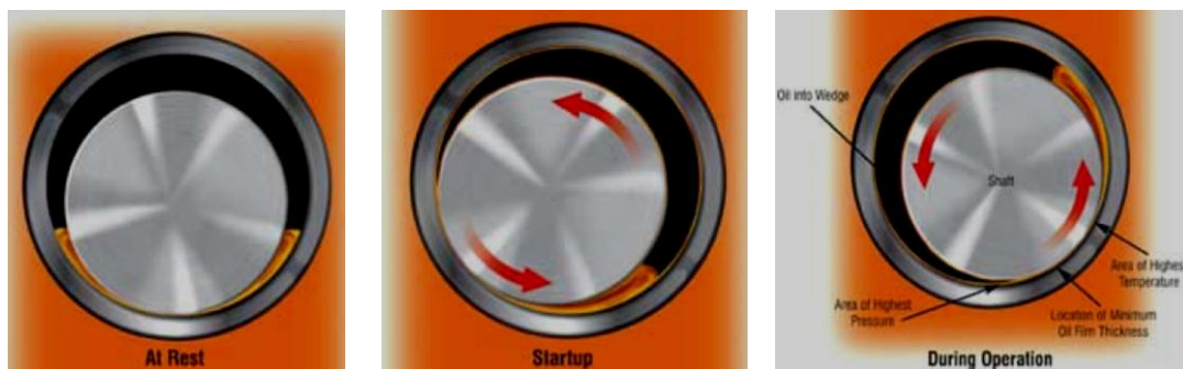
Gambar 2.5 Posisi bearing saat diam, permulaan awal dan operasi normal [3]
