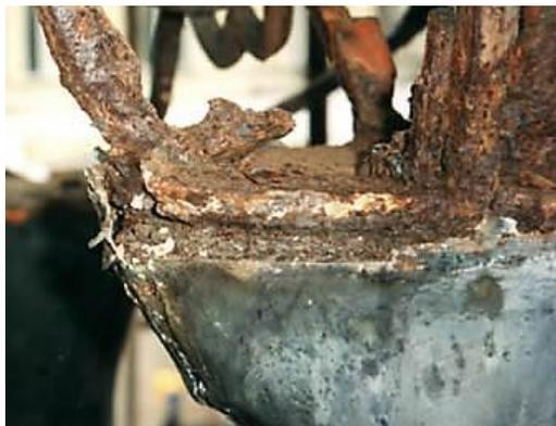
**Gambar 2.11.** External corrosion damage factor-ferritic component [23].
