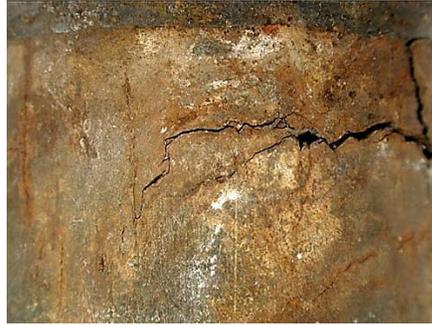
**Gambar 2.9.** *Sulfida stress cracking* [21].
