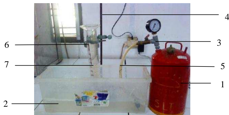
Gambar 3.4. Water Displacement Technique
