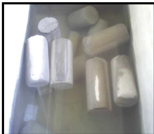
Gambar 3.9. Proses perawatan ( curing ) benda uji
