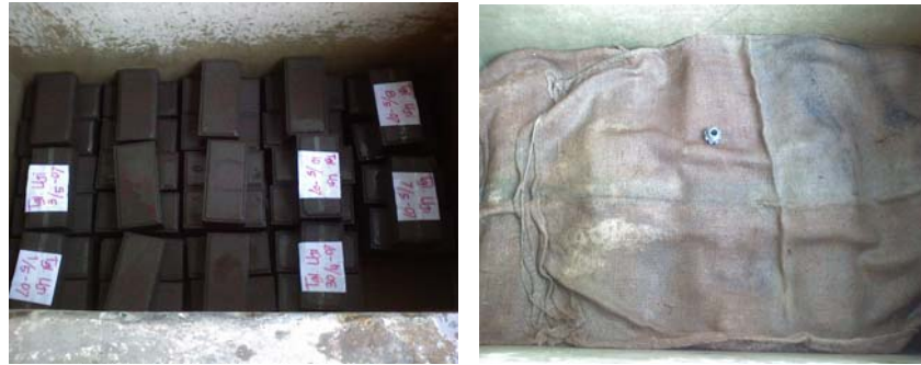
Gambar 3.2 Perawatan Paving Block
