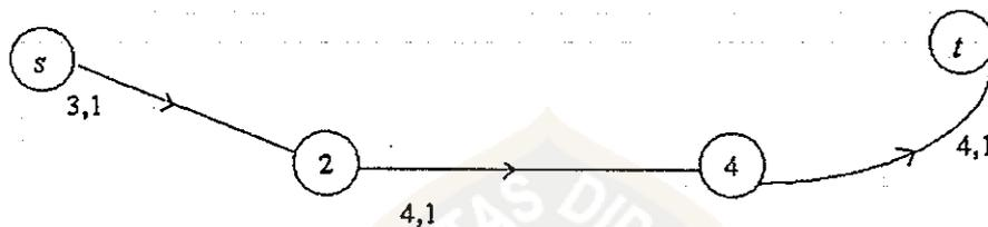
Gambar 2.12. Ilustrasi *flow augmenting path*
