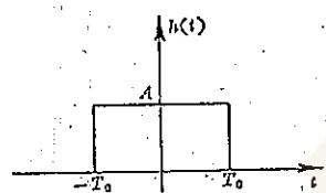
$$h(t) = \begin{cases} A, & |t| < T_0 \\ \frac{A}{2}, & |t| = T_0 \\ 0, & |t| > T_0 \end{cases} \Leftrightarrow H(f) = 2AT_0 \frac{\sin(2\pi f T_0)}{2\pi f}$$
