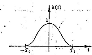
$$h(t) = \begin{cases} \frac{1}{2} + \frac{1}{2}\cos\left(\frac{\pi t}{T_0}\right), & |t| \leq T_0 \\ 0, & |t| > T_0 \end{cases}$$
