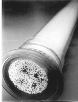
Gambar 2.7 Modul membran *Hollowfiber* (Coulson and Richardson, 2002)
